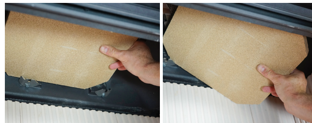
Removal of the upper deflector plate. (HKD 13)
