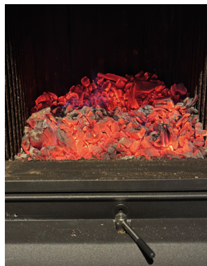
Ember bed without flames - burning finished
