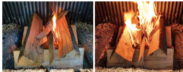
Perfect lighting process in the firing bowl of the combustion chamber with lighter and fire-starter between the top layer of wood logs.
