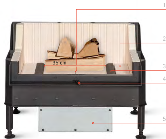
1 Combustion chamber floor with integrated firing bowl 2 Side floor stones 3 Side combustion air inlet (primary air) 4 Combustion air adjusting lever 5 Connection box for the air intake flap of the combustion control system
