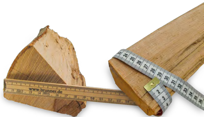
A log circumference of 25 cm corresponds to a log diameter of about 9 cm
