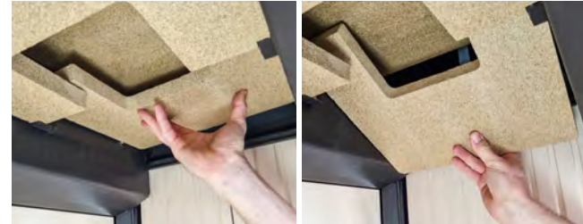
Removal of lower deflector plates
